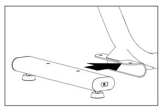
Figure 2: Rear stabilizer installation
